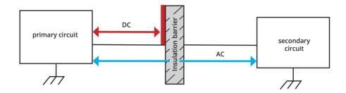
This isolation barrier significantly reduces or prevents interference and damage in electrical systems that could otherwise be caused by various factors, such as potential differences, surges, noise or ground loops. Another important factor is the protection of persons from electric shock.
